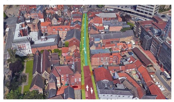
A proposed concept of how an alternative true pedestrian/cycle street could work, with widened footpaths (green), a distinct cycle lane (blue) and bi-directional vehicle access to the south (red).
